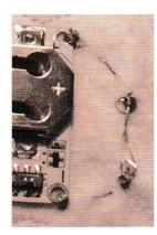
Sew the other LED into position repeating steps 11 - 14. Make sure you use a new piece of thread each time you stitch a new section of the circuit. Push a cell (battery) into the cell holder and switch it on to test your circuit works. The on/off switch is the tiny black switch on the surface of the cell holder which slides backwards and forwards.
